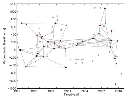
Figure 2: Timeline-baseline plot showing the SAR master scene (black) and the interferogram network generated by combining a number of ERS SAR images (red). The gray dots correspond to unused SAR scenes that resulted in no or low interferometric correlation.
