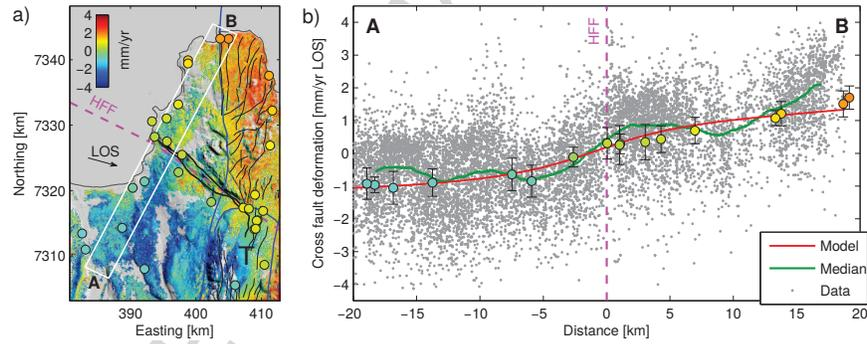
Figure 5: a) LOS InSAR and GPS (filled circles) displacement rates in map view. Bold lines mark HFF fault traces and the model segments are indicated in purple. b) GPS (circles with error bars) and InSAR (gray dots, purple line) in comparison to the model prediction (red line). The data have been corrected for volcanic inflation at Theistareykir (T) using the Mogi model parameters from Metzger et al. (2011).
