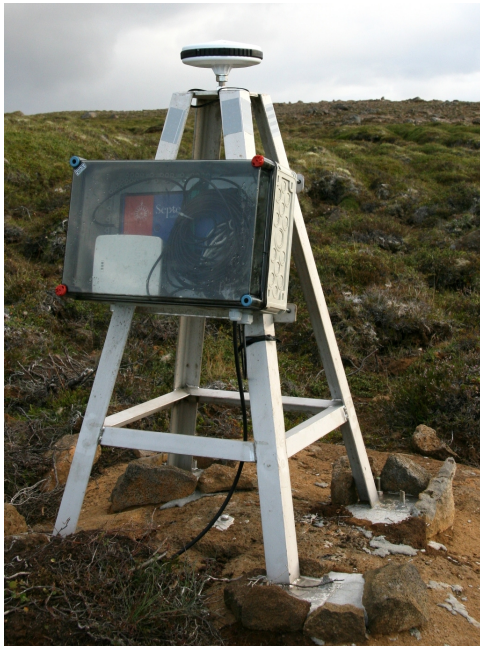
Figure 2. Example of a set up for the continuous GPS stations in North Iceland. The stainless-steel quadri-pod of the station SAVI is drilled and cemented into the ground. The box protects the GPS receiver and the wireless LAN antenna, which is used for data transmission to an Internet access in 6 km aerial distance.
